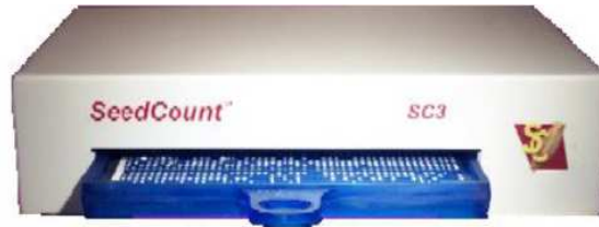
Figure 1: (b). Seed Count Tray in Scanner Cabinet (Armstrong et al. 2005)
